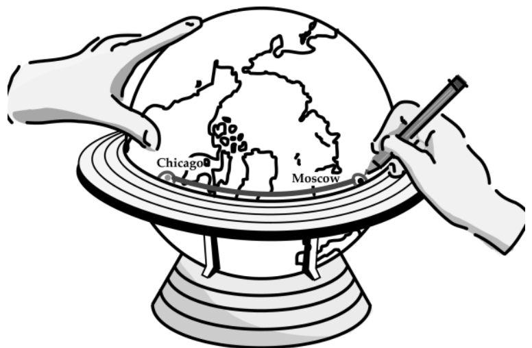
Step 4 Draw a line, using the Horizon Ring as a straight edge connecting the two cities.
